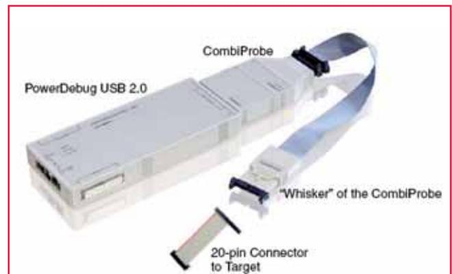
Fig. 1 - Sistema TRACE32 PowerDebug USB CombiProbe
