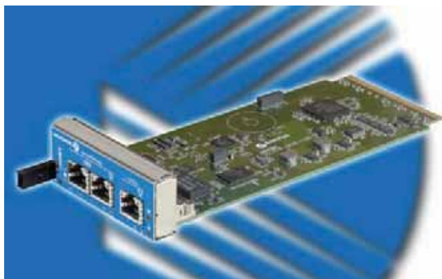
Fig. 3 - Il Management Controller Hub (MCH) AM4901
