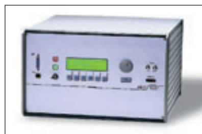
Fig. 4 - Load dump Generator PG2800 (Hilo test)
