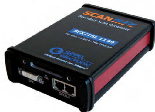
Fig. 4 – Hardware - Boundary Scan controller di GOEPEL electronic (SFX-TSL1149.x)
