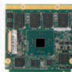
**Q7-BW****Qseven® Standard Size Module with Intel® Pentium™ and Celeron™ Processor N3000 Series SoC**
