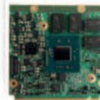
**Q7-BT****Qseven® Standard Size Module with Intel® Atom™ Processor E3800 Series SoC**
